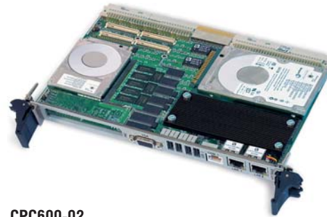
CPC600-02 HDD 1.8" site, HDD 2.5" site, reduced heat sink
