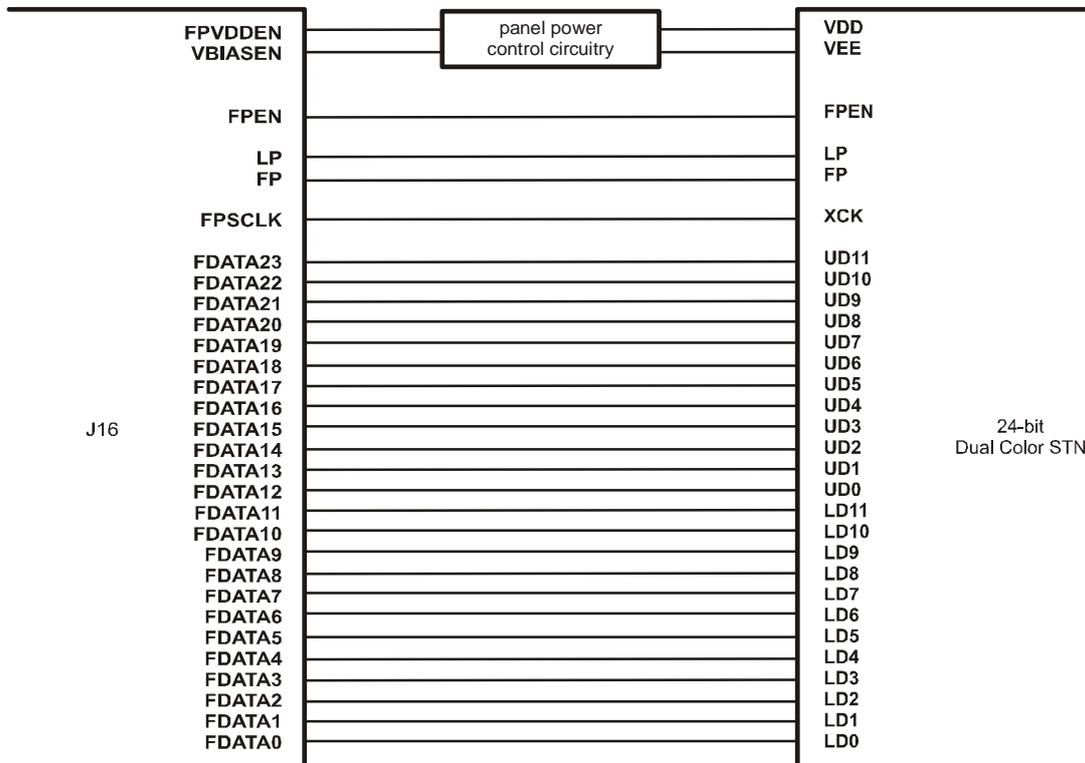
Figure 4.8: Connection of a TFT Panel with 1 Pixel per FPSCLK Period
