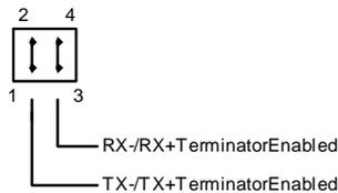
To use any of the COM3 – COM6 ports in RS-422 or RS-485 mode, do the following:
