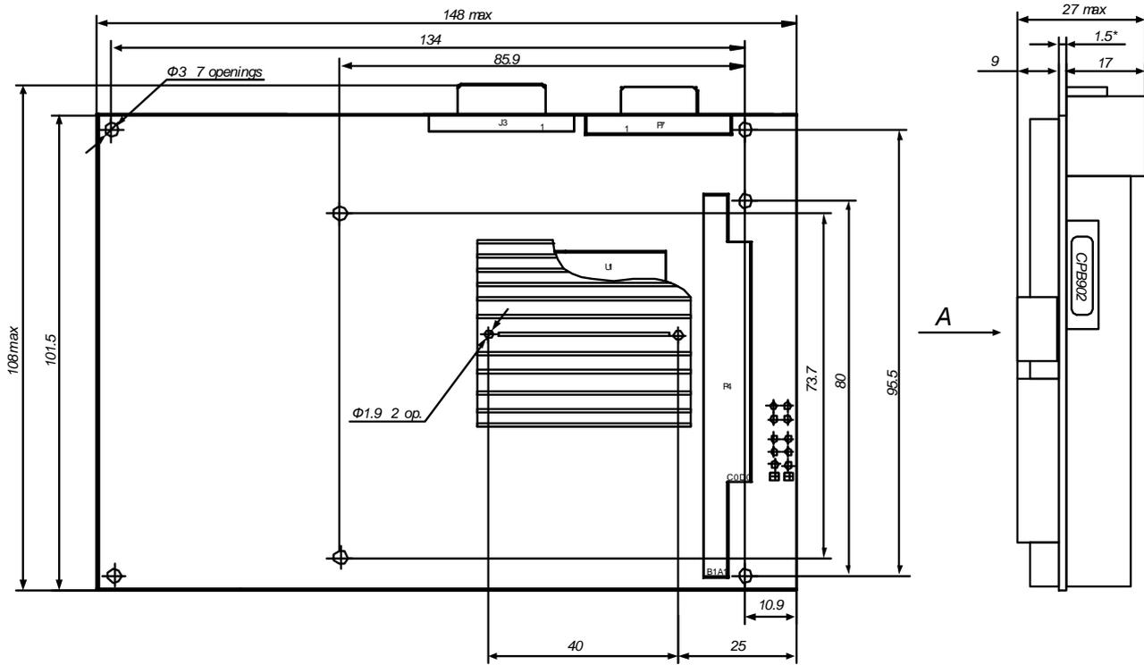
Figure 4.32: CPB902 Bottom Side: Overall and Mounting Dimensions
