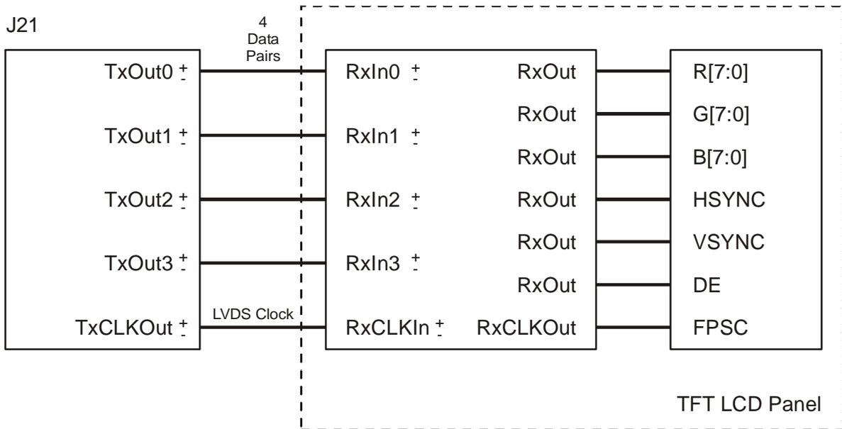
Figure 4.11: PanelLink Interface for TFT LCD Panel
