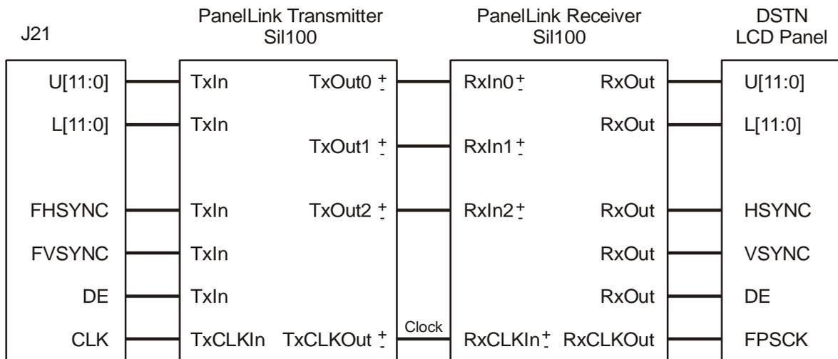
Color DSTN panels with 16-bit or 24-bit interface and resolutions up to 1280x1024 and 1024x768 respectively are supported. For color TFT panels the color resolutions of 9, 12, 18, and 24 bits per pixel are supported.
