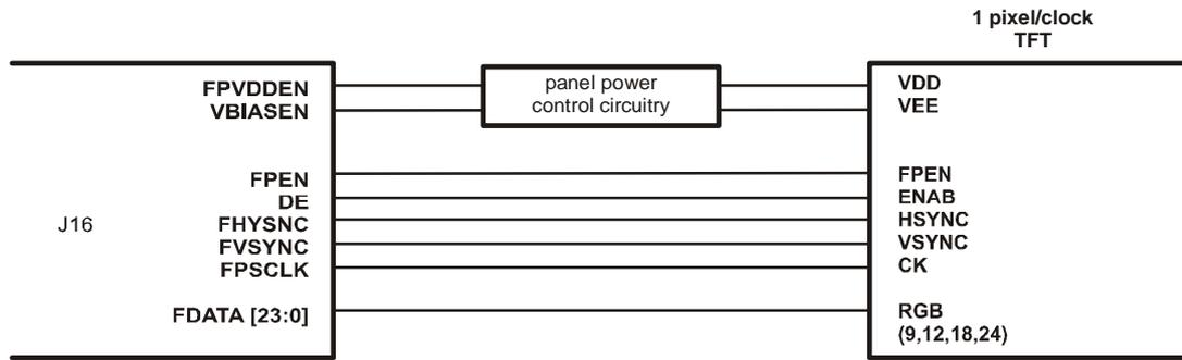
Figure 4.9: Connection of a TFT Panel with 2 Pixels per FPSCLK Period
