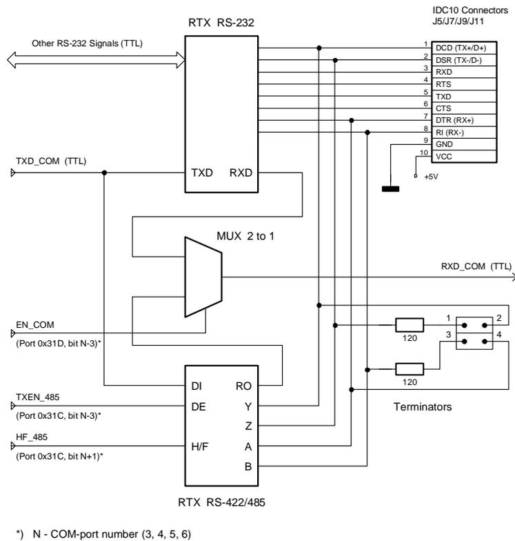
In RS-232 mode the terminators should not be enabled. In RS-485 or RS-422 modes the jumpers should be set on appropriate pinpads: J6 (COM3), J8 (COM4), J10 (COM5) and J12 (COM6). In RS-485 mode jumper 1-2 should be set on terminating modules; in RS-422 "point-to-point" mode jumper 3-4 should be set. Switching to RS-422/RS-485 modes is done in BIOS Setup. For COM1 – COM6 ports base addresses, please, refer to Tables 4.2 and 4.3.
