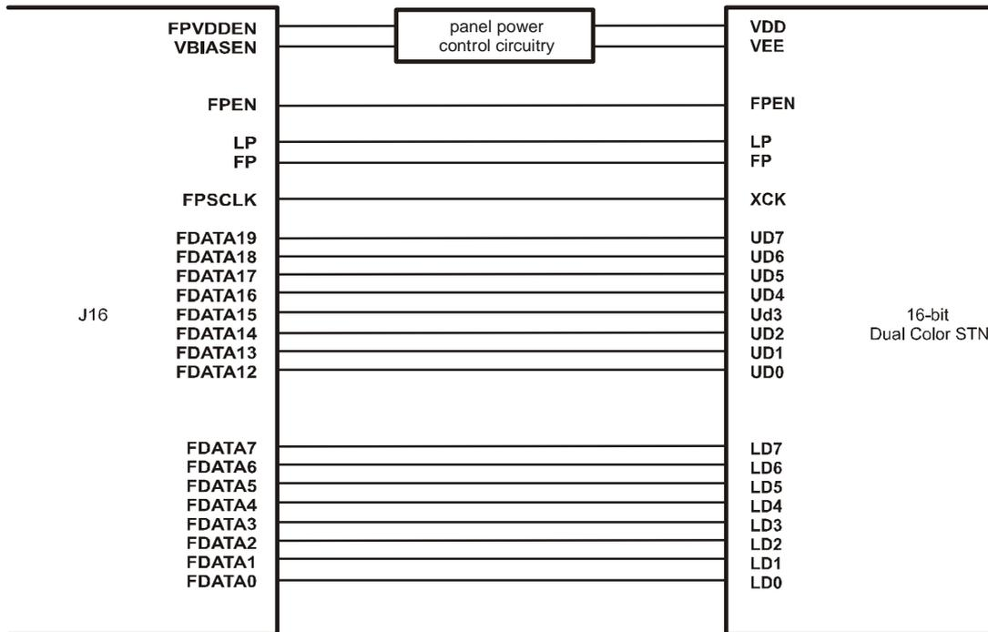
Figure 4.7: Connection of 24-bit DSTN Panel
