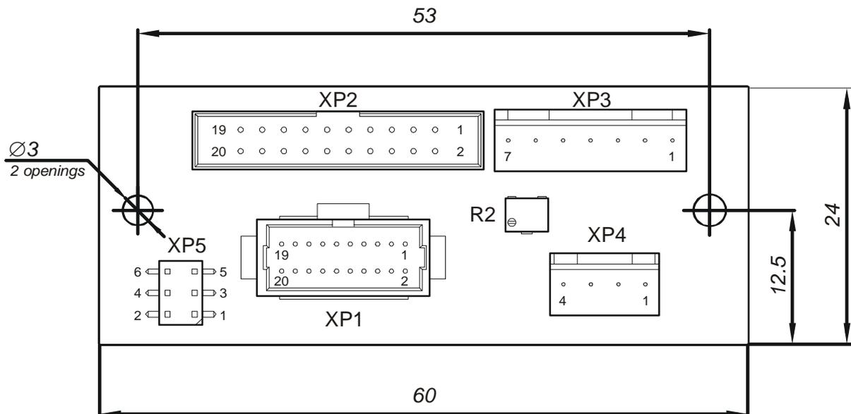
Figure 4.15: CVM04 Connections Diagram
