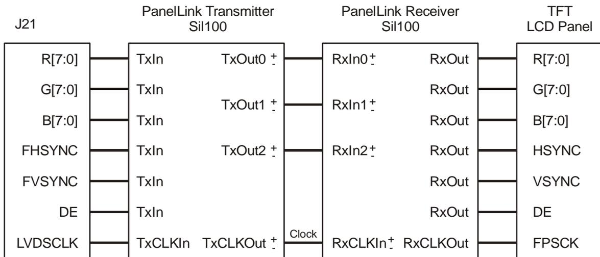
**Figure 4.12: PanelLink Interface for DSTN LCD Panel**
