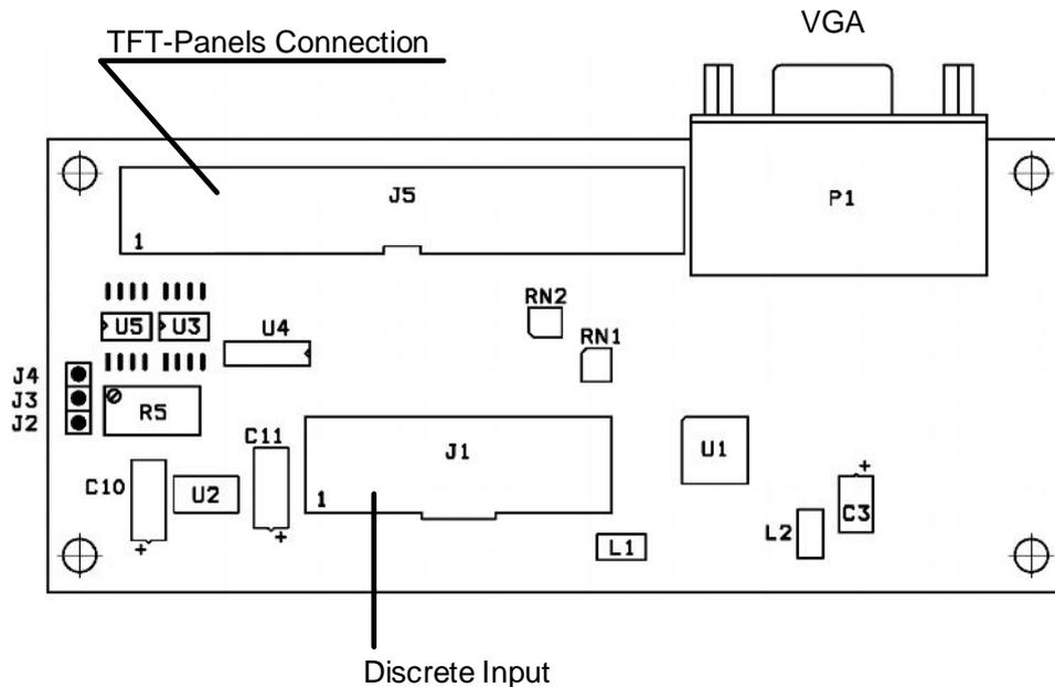
The CVM01 P1 VGA connector has the same pin assignments as CPB902 P7 connector (see [P7 Pinout Table](#) in subsection 4.3.7.1). The pinout of CVM01 J5 connector is given in the table below.
