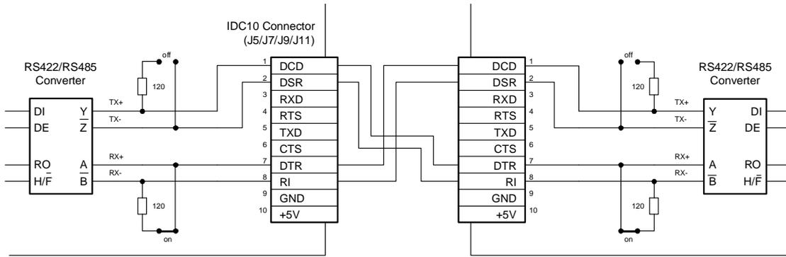
**Figure 4.21: Connection of Several Devices in RS-485 Mode**
