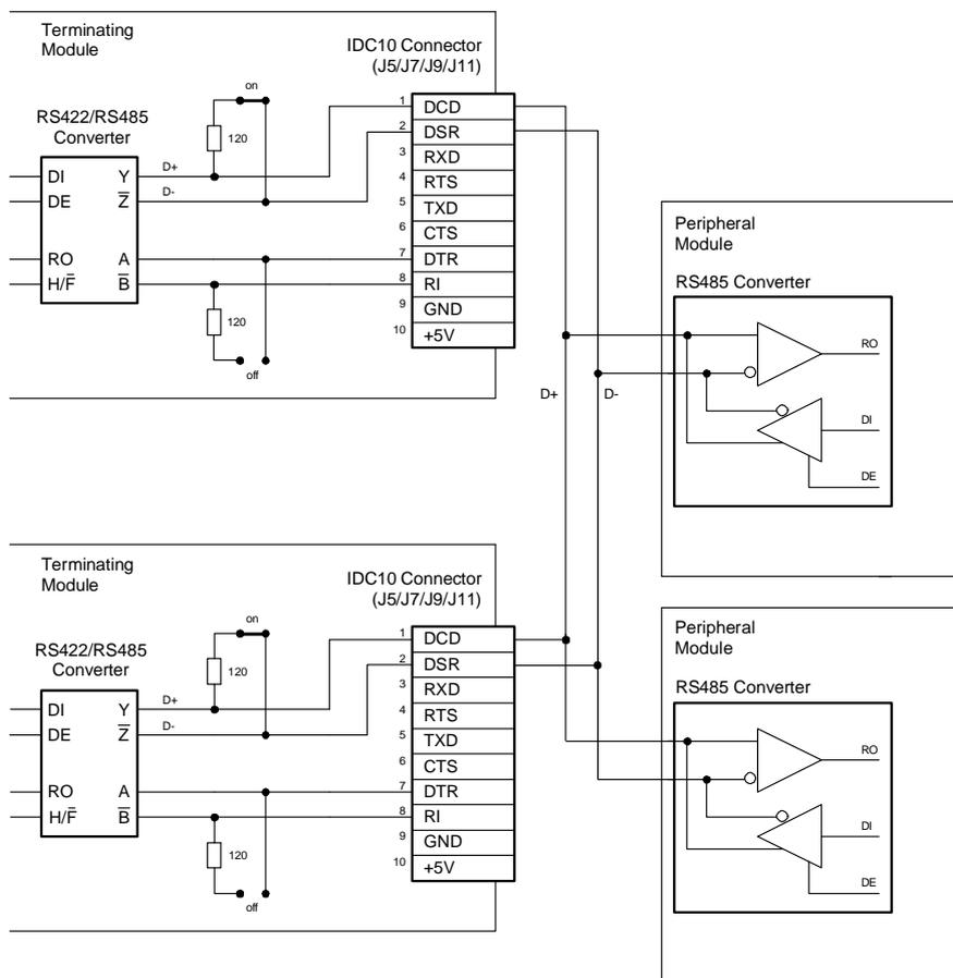
Figure 4.22 presents a diagram explaining functioning and mode selection for one of COM3 – COM6 ports.
