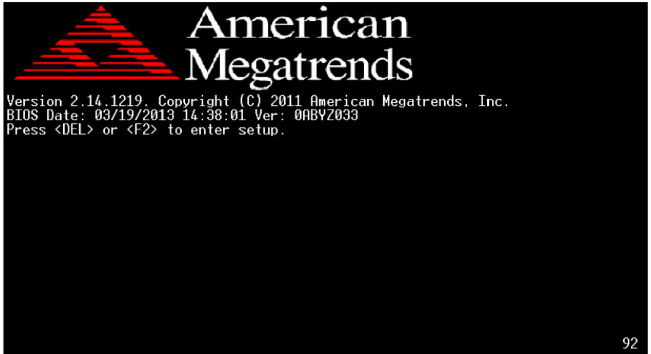
Using the BIOS Setup Utility program, it is possible to change parameters of BIOS (Basic Input Output System) and control special operation modes of the module. This program uses menu system for introducing changes, as well as for switching on or switching off special functions.
