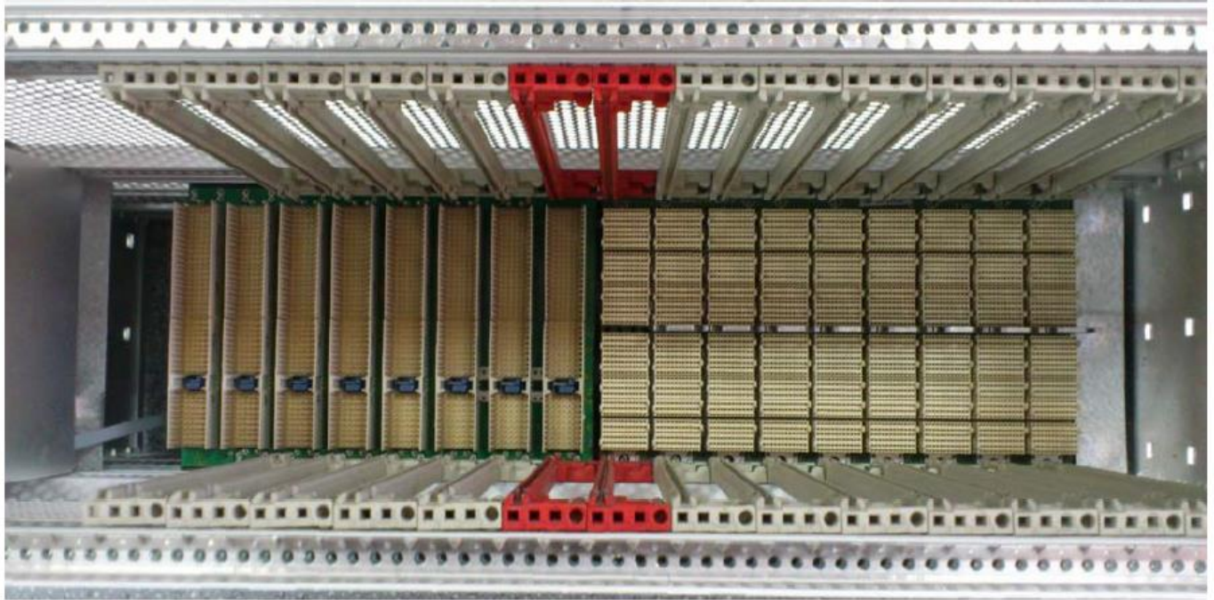
Fig. 3-12: Example of the assembled backplanes in the extended hybrid system
