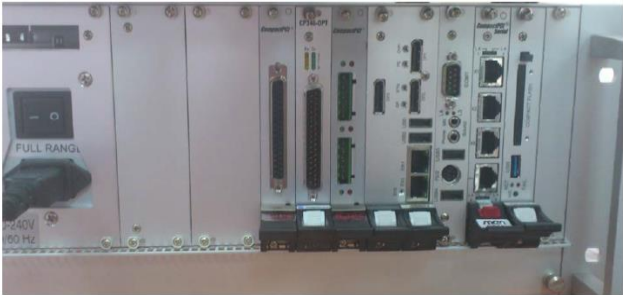
Fig. 3-10: Example of system generation on the basis of PICMG 2.30 backplane (Plus I/O) and CPC510-02 CPU board
