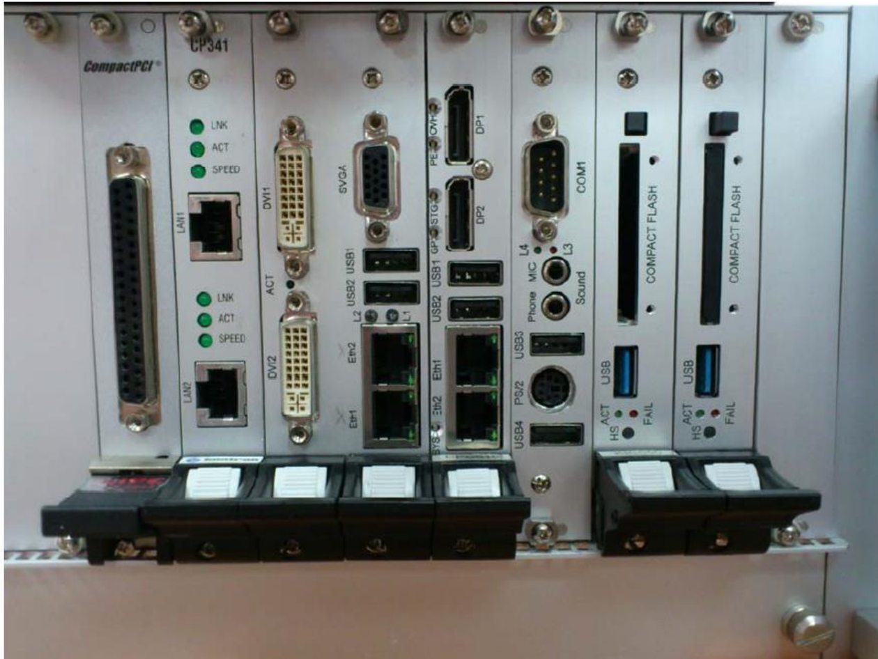
Fig. 3-11: Example of PICMG 2.30 system generation with the main CPC506-03 CPU board and additional on-board CPC510-01 computing device
