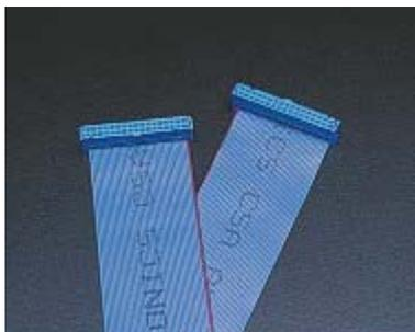
The FC cables are used to connect control and expansion cards to external I/O peripherals. There is an IDC connector on both ends of each cable. The first number following "FC" is the number of conductors, and the second number is the length in centimeters.
