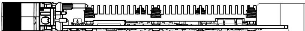
Fig. 1-10: CPC512 module with the installed copper R1 4HP heatsink (side view)
