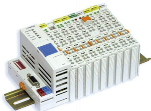
The modules ensure connection of sensors and actuators, and also contain galvanic isolation and status indication circuits. The modules are powered via the internal bus by the integrated controller source or additional power supply modules.
