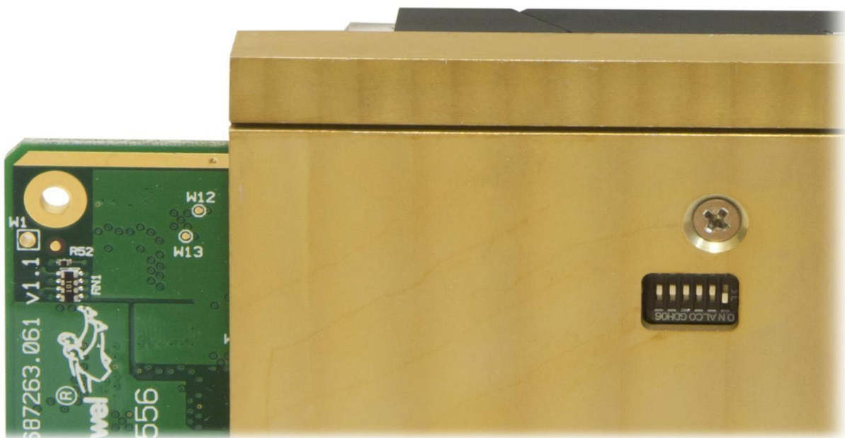
Fig. 4-2: Switch of operating modes of VIM556RC (SA1)
