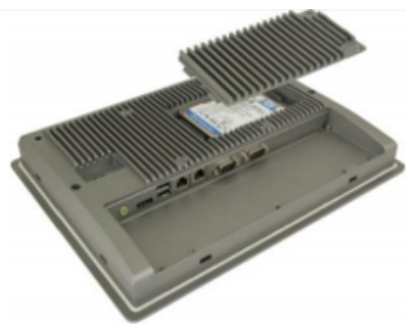
Access to SSD/HDD
