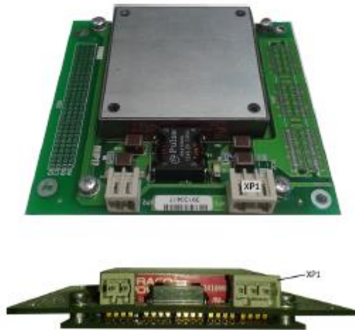
Fig. 3-4: Photos of the module showing the location of the XP1 power supply connector
