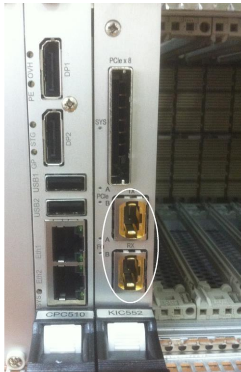
Fig. 3-7: Connectors for optical cables with the removed stopping plugs
