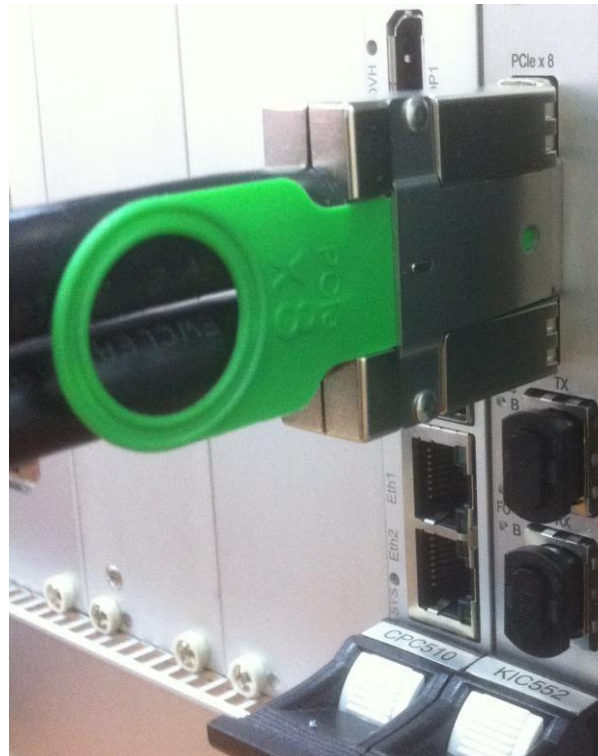
Fig. 3-2: Cable PCI Express External Cabling x8, connected to KIC552 module
