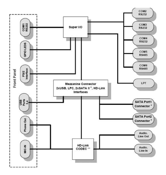
\* SATA connectors are provided only for MIC584-01 version (Fastwel manufactures MIC584 in two versions: MIC584-01 and MIC584-02). \*\*Audio controller for module version 2.1: AD1986A, for version 3.1: CS4702.
