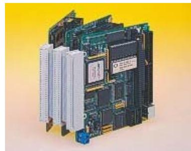
The FC62-2 (MK20) and FC62-3 (MK-30) flex backplanes can stack two or three computer cards together. These flexible backplanes are ideal in limited space applications. Moreover, they ease service operations.
