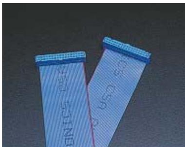
The FC cables are used to connect control and expansion cards to external I/O peripherals. There is an IDC connector on both ends of each cable. The first number following "FC" is the number of conductors, and the second number is the length in centimeters.
